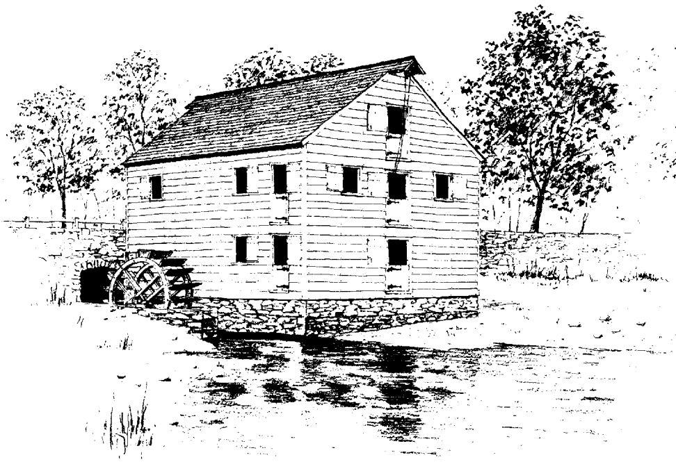
Robeson-Williams Grist Mill (1715–1740). Conjectural drawing showing original appearance of the mill. Water wheel should be of “over-shot” type.
